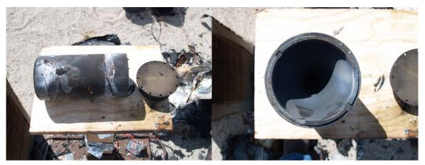
Figure 6. Photographs of the Shaped Charge After the Cook-off Test (No damage to the liner or body was evident)
