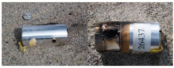
Figure 3. Photographs Showing the Entrance and Exit Holes from the Bullet Impact Test
