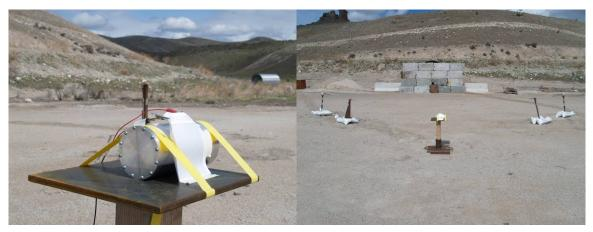
Figure 2. The 3.2-inch Generic Shaped Charge Prepared for Bullet Impact Test
